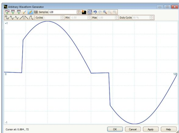
A function generator is also included, with sine, square, triangle, DC level and many more standard waveforms. As well as level, offset and frequency controls, advanced options allow you to sweep over a range of frequencies. Combined with the spectrum peak hold option, this creates a powerful tool for testing amplifier and filter responses.
