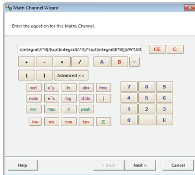
With PicoScope 6 you can perform a variety of mathematical calculations on your input signals and reference waveforms.
