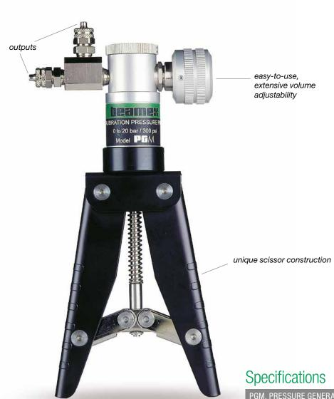
**The PGM** is a hand-operated pressure calibration pump that uses air as its pressure medium. The extremely accurate volume control provides the excellent fine adjustment of pressure. The pump's unique and sturdy construction makes the PGM the ultimate field calibration pump.
