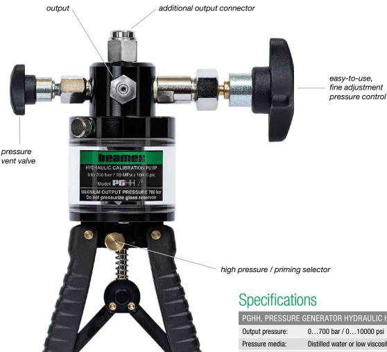
**The PGHH** is a hand-operated, hydraulic, high-pressure generator compatible with different liquids (e.g. mineral oil, distilled water, etc.). The pump is equipped with an adjustable volume control for fine-tuning generated pressure. PGHH also includes a prime/high stroke selector for easy use.
