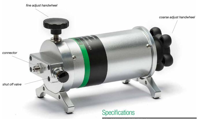
**The PGL** is a hand-operated pressure table pump for low pressure using air as its pressure medium. The pump is equipped with an isothermal bellows chamber for reducing possible environmental temperature changes during the calibration process. With the screw-operated volume control and fine adjustment, an extremely accurate and stable pressure adjustment is possible.
